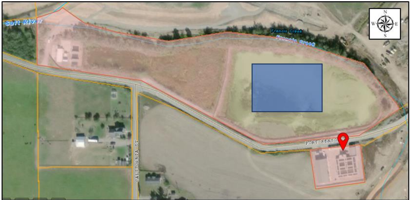
Figure 5 Image of the available installation area (in blue) for a floating solar array at Ferndale's WWTP, meter location marked in red.
